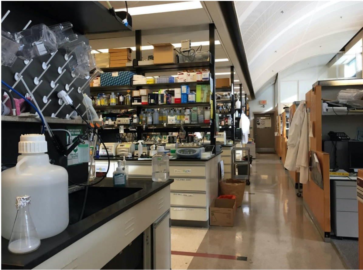
Figure 3. View of an occupied lab, showing lab modules at left and workstations on the window wall at right. The higher ceiling over the workstations was made possible by stopping the interstitial service floors above the lab modules, rather than extending them to the exterior wall. Source: Author.
