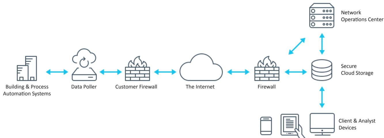
Figure 2: Automated building analytics network architecture
