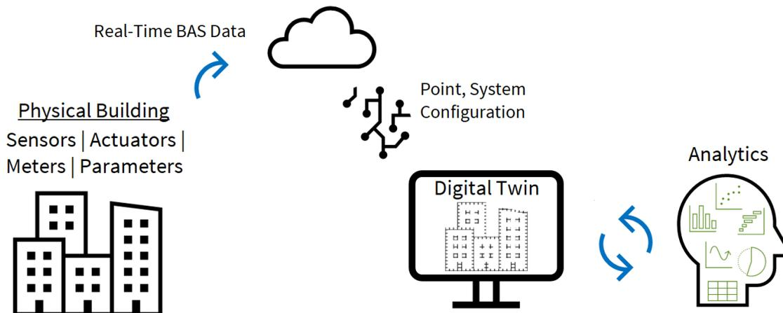
Figure 1: A representation of the Digital Twin model. All images in this guide ©Cimetrics Inc. Analytica 2020
